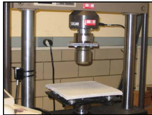
Figure 2: Punching Shear Test
