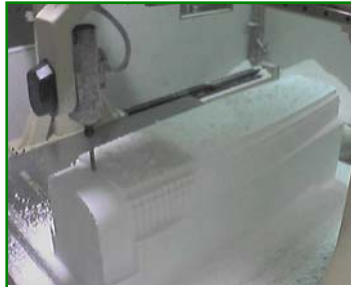
Figure 4 – Milling of Plug
