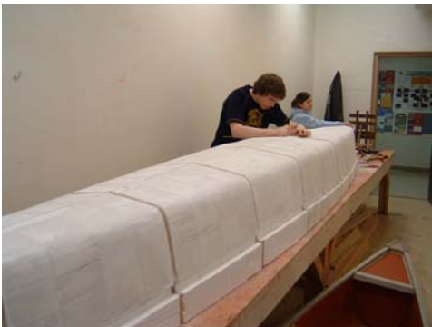
Fig. 4: Foam and plywood cross-sections
