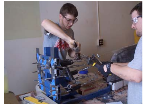
Fig. 5: Tensioning of the prestress wires
