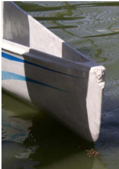
Fig 1: Damage to the bow of Cerulean (note the scrapes at the bottom)
