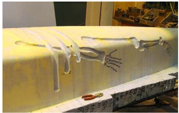
Figure 6 Aesthetic reliefs on the canoe mold.
