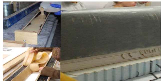
Figure 8 : Polyurethane gauges for the gunwales
