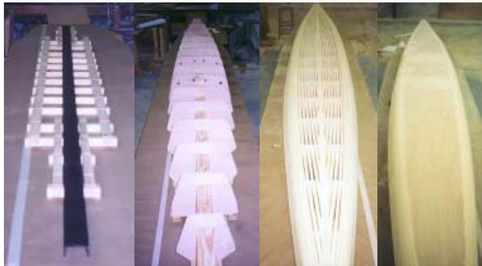
Figure 6.1: The sequential order that the form was constructed
