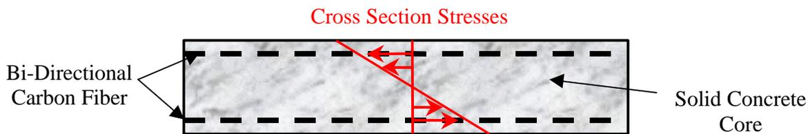
**Figure 5. Reinforcement Scheme with Stresses**
