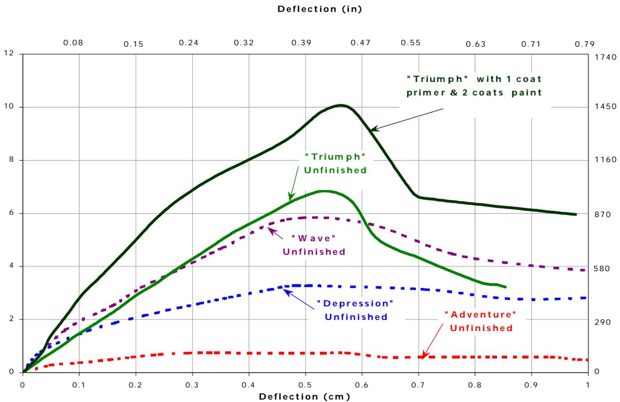
Figure 6. Flexural Test Results on Finished and Unfinished Test Plates (14 Day)
