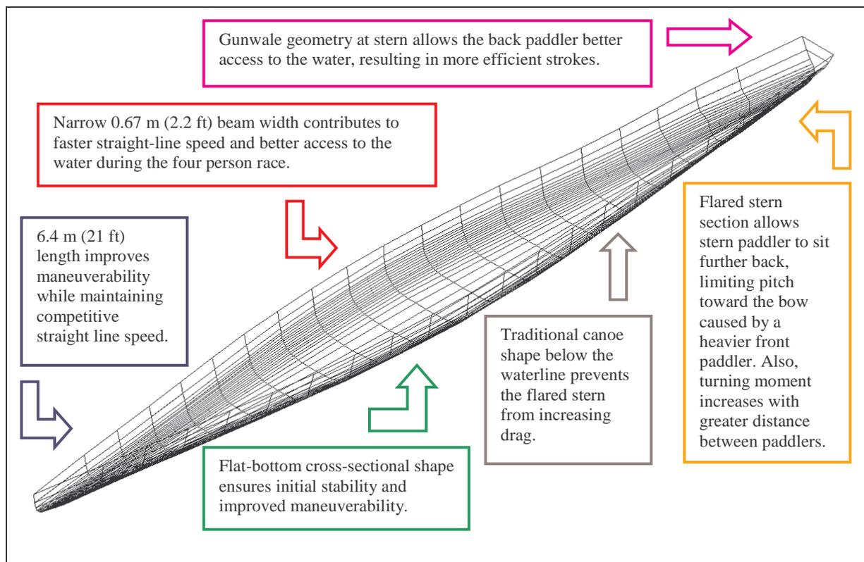
Figure 1: **CALCATRAZ** Hull Design
