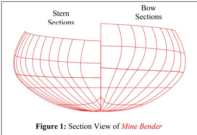
**Figure 1:** Section View of *Mine Bender*
